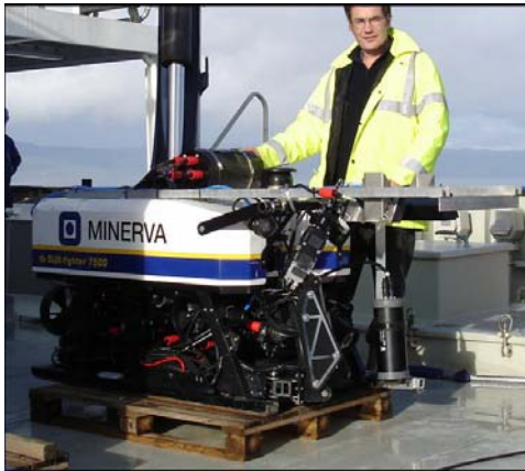
GeoSwath mounted on a Minerva ROV shown with 500 kHz ROV transducers
